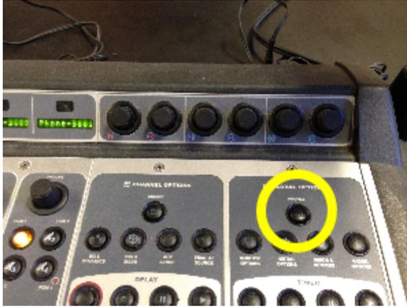
The Profile button shows the available profiles on the soundboard screen, and you can use the F1 knob as in “Changing Sources.”
