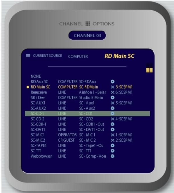
5. Scroll again using the F1 key to hover over the source you want. In this case, the channel currently has “RD-Main” (Rivendell output) selected and we’re selecting the CD1 player. Pressing the F1 knob will select the source illuminated in the greenish-gray box.
